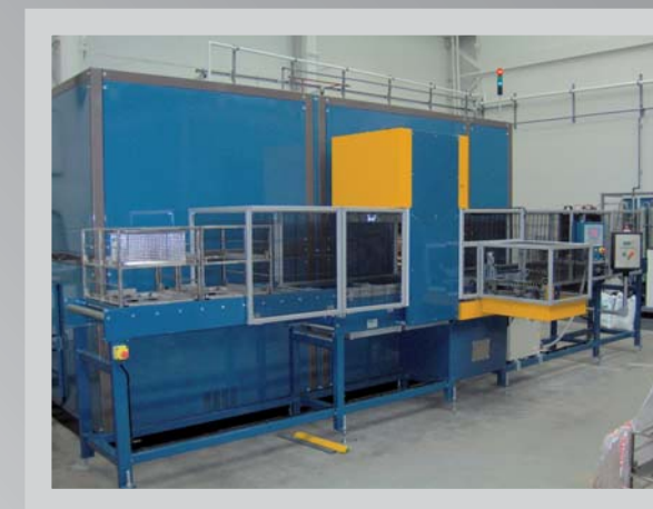
MUMV 100 Metal degreasing systems using Dowcylene 1601 solvent under vacuum Automatic loading system
