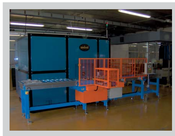
MDMV 2 Metal degreasing systems using chlorinated solvents under vacuum Automatic loading system
